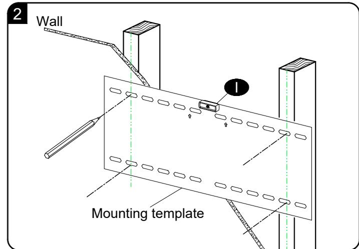
3. Drill pilot holes using a 1/8 in. (3 mm) diameter drill bit.
