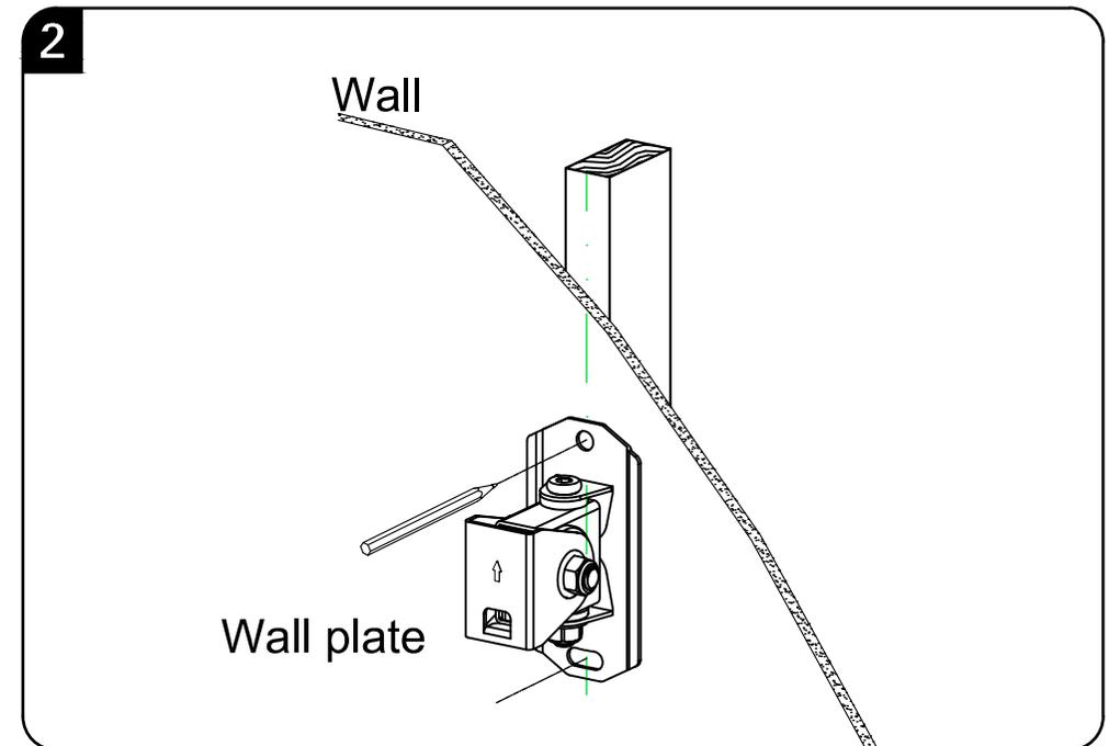
3. Drill pilot holes using a 1/8 in. (3 mm) diameter drill bit.
